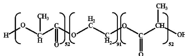
Fig.1 Triblock-copolymer of poly-L-lactide and poly (ethylene glycol).
