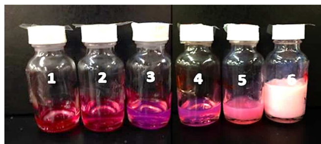
Figure 1. Representative, normalized, SEC traces for the PSMA 19 - b -PPPMA y series of AB diblock copolymers prepared in n -octane and digital pictures of the RAFTDP solutions at 20 °C for an \bar{X}_n of PPMA of (1) 31, (2) 57, (3) 75, (4) 88, (5) 101 and (6) 131.
