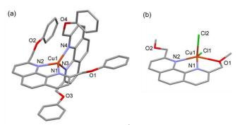
**Fig. 4** Molecular structures of (a)  $[Cu^{l}(4)_{2}]^{+}$  (the PF<sub>6</sub><sup>-</sup> anion is omitted for clarity) and (b)  $[Cu^{l}(5)Cl_{2}]$ . Selected bond lengths (Å) and angles (deg) for  $[Cu^{l}(4)_{2}]^{+}$ : Cu1–N1 2.029(2), Cu1–N2 2.038(3), Cu1–N3 2.048(3), Cu1–N4 2.032(3); N1–Cu1–N2 82.1(8), N3–Cu1–N4 82.2(7), N1–Cu1–N3 123.5(7), N2–Cu1–N4 132.8(8); for  $[Cu^{ll}(5)Cl_{2}]$ : Cu1–N1
