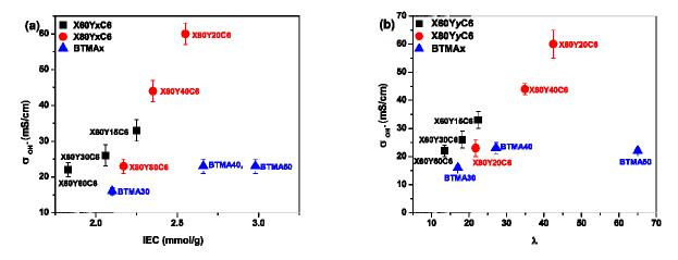
Figure 4. Hydroxide conductivity of membranes as a function of (a) IEC (ion exchange capacity) and (b) hydration number  $\lambda$  (moles of water per mole of quaternary ammonium group) in water at room temperature. Conductivities were measured with samples exposed to liquid water.
