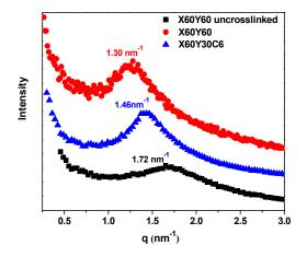
Figure 6. SAXS profiles of dry polymer membranes in the bromide form.
