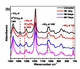
Figure 9. ATR spectra of treated X60Y15C6 membrane (a) ATR spectra of functional group region (b) fingerprint region.
