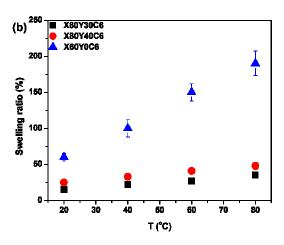
Figure 3. Liquid water uptake (a) and swelling ratio (b) of membranes in OH form as a function of temperature.
