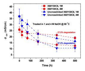
Figure 8. Chemical stability of the quaternary ammonium cation of X60Y30C6 and uncross-linked X60Y30C6 in 1 M and 4 M NaOH solution at 80 °C, and OH conductivity as a function of duration time measured at 20 °C.
