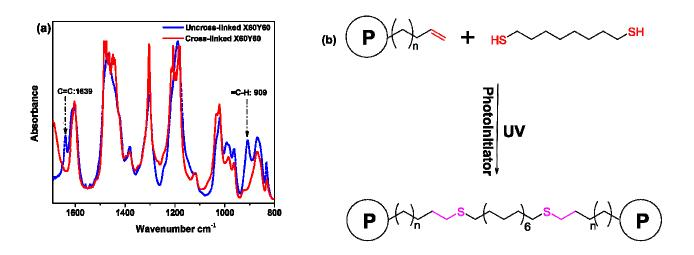
Figure 1. FTIR spectra of uncross-linked and cross-linked membranes (a) and schematic plot of cross-linked reaction (b).
