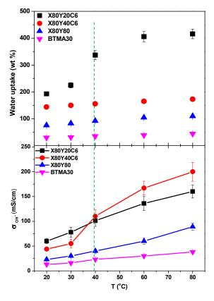
Figure 5. Hydroxide conductivity of X80YxC6 and BTMA30 membranes as a function of temperature. Conductivities were measured with samples exposed to liquid water.
