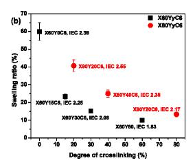
Figure 2. Liquid water uptake (a) and swelling ratio (b) of membranes in OH<sup>-</sup> form as a function of degree of cross-linking at room temperature.
