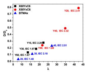
Figure 7. Ratio of the diffusion coefficient, D, to the dilute solution diffusivity,  $D_0$ , as a function of hydration number for membranes in the hydroxide form.
