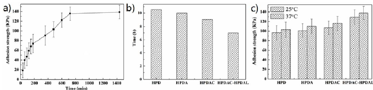
Fig. 7 (a) Time-Adhesion strength curves of HPDAC-HPDAL. (b) Respectively the time of copolymers when adhesion strength was 100 KPa at 37 °C. (c) The adhesion strength of copolymers respectively at 20 °C and 37 °C after 12 h.
