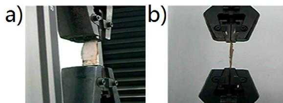
Fig. 1 (a) Positive of pork skin in the test process. (b) Side of pork skin in the test process.
