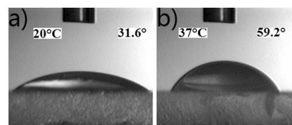
Fig. 4 Photographs of water droplet shape and contact angle on the film surface of polymer at 20 °C and 37 °C.
