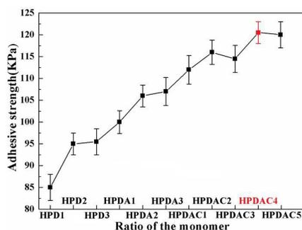
Fig. 2 Ratio of copolymeric monomer-Adhesive strength curves after 24h at 37 °C.
