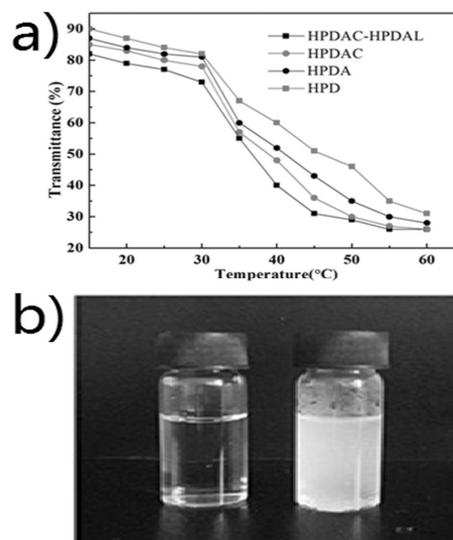
Fig. 3 Temperature-sensitive test results (a) Temperature-Light transmittance curves of HPD, HPDA, HPDAC, HPDAC-HPDAL. (b) HPD aqueous solution (0.3 mg/mL) respectively under 20 °C and 37 °C.
