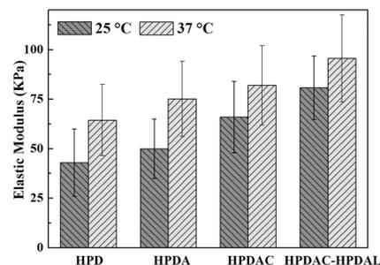
Fig. 6 The elastic modulus value of copolymer was also evaluated at 25 °C and 37 °C after 12 hours of reaction.
