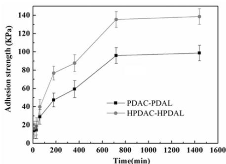
Fig. 8 Time-Adhesion strength curves of hyperbranched and linear polymers under 37 °C.
