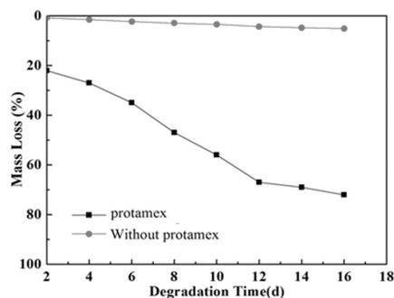
Fig. 9 Time-Mass Loss curves of HPDAC-HPDAL under 37 °C.
