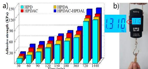
Fig. 5 (a) Time-Adhesive strength relation of the different copolymers under 37 °C.
