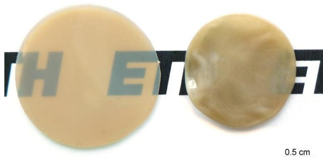
Figure 3: Compression moulded film with a thickness of 0.6 mm before exposure to acid (left) and after treatment with TfOH for 60 min (right). Besides the considerable shrinkage the overall shape of the film is largely retained while the transparency vanishes.
