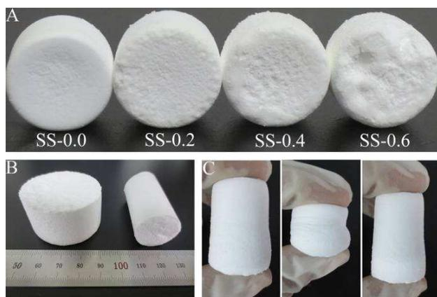
**Fig. 1** Digital images showing the macroscopic properties of sponge (A: Sponge prepared with various amount of TEOS; B: Two monolithic sponges of SS-0.2 with different dimensions; C: A bulk sponge of SS-0.2 was compressed and recovered to the original volume quickly by finger tips).
