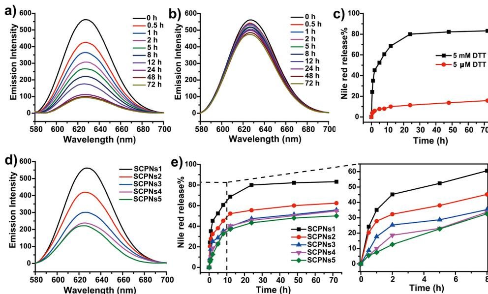
**Fig. 8** Nile red release from SCPNs1 in response to varied DTT concentration, (a) 5 mM, (b) 5  $\mu\text{M}$ . (c) Comparison of Nile red release rate from SCPNs1 under different concentration of DTT. (d) The emission spectra of Nile red sequestered in SCPNs1-5. (e) Comparison of DTT-induced Nile red release rate from SCPNs1-5.
