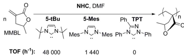
Scheme 6. Polymerization of MMBL using different NHCs [21].
