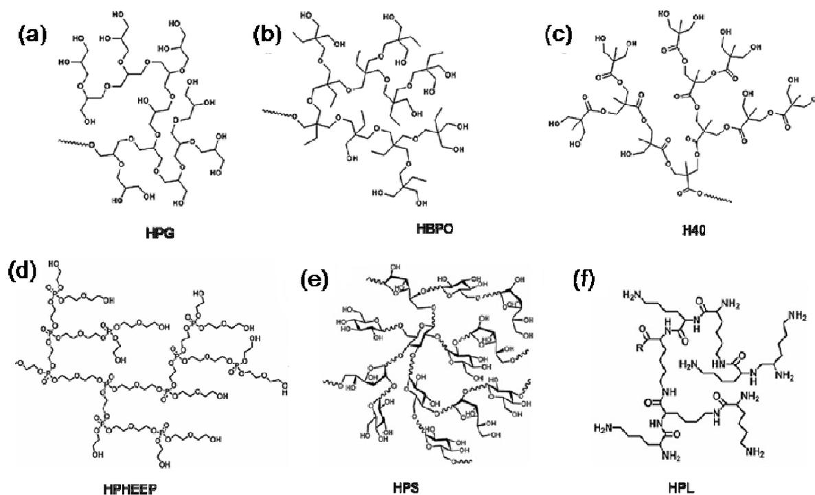
**Fig. 1** Schematic structures of representative biocompatible or biodegradable HBPs: (a) hyperbranched polyglycerol (HPG), (b) hyperbranched poly(3-ethyl-3-oxetanemethanol) (HBPO), (c) hyperbranched polyester (Boltorn<sup>®</sup> H<sub>40</sub>), (d) hyperbranched polyphosphate (HPHEEP), (e) hyperbranched polysaccharide (HPS), and (f) hyperbranched polylysine (HPL). Reproduced from ref. 10. Copyright 2014 Royal Society of Chemistry.
