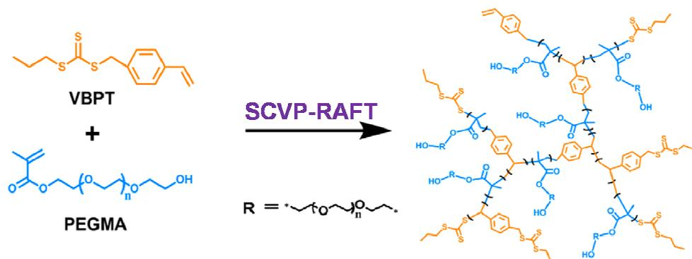
**Fig. 4** A schematic illustration of hyperbranched poly(VBPT-co-PEGMA) constructed by SCVP-RAFT using VBPT and PEGMA monomers. Reproduced from ref. 68. Copyright 2014 American Chemical Society.
