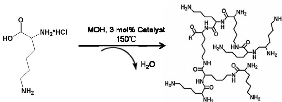
**Fig. 2** A schematic illustration of hyperbranched polylysine constructed by the SGP of *L*-lysine monomers. Reproduced from ref. 48. Copyright 2007 Wiley-VCH.
