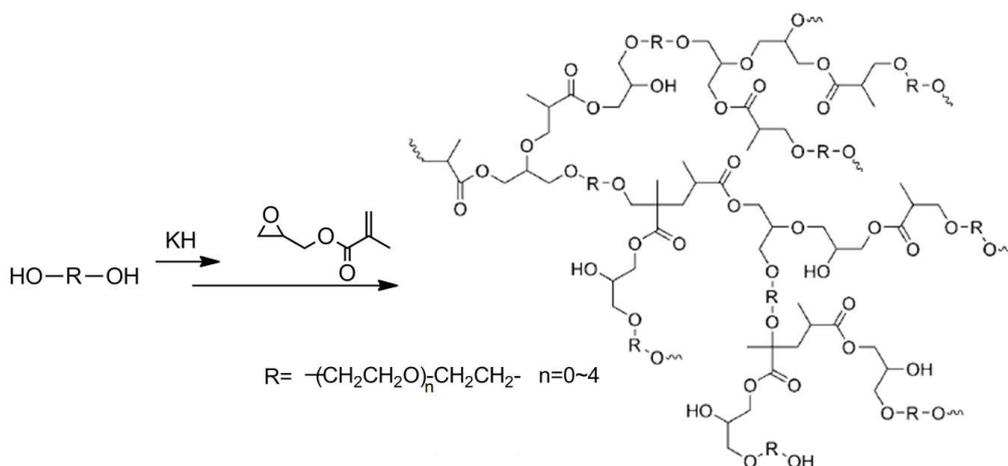
**Fig. 6** A schematic illustration of the simultaneous vinyl polymerization and ring-opening
