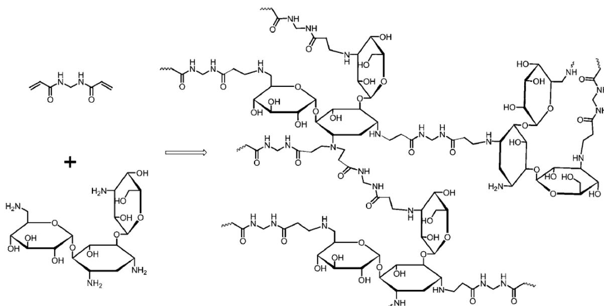
**Fig. 3** A schematic illustration of hyperbranched polysaccharide constructed by SGP using *N,N'*-methylene bisacrylamide and kanamycin monomers. Reproduced from ref. 56. Copyright 2011 Royal Society of Chemistry.
