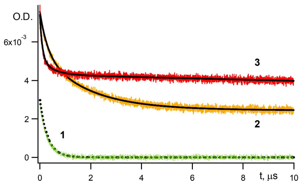
**Fig. 2.** Kinetics of  ${}^3\mathbf{B}^*$  measured at  $\lambda$  630 nm at 263 K obtained under laser flash photolysis of **B** in **E** film (1); decay kinetics of  ${}^3\mathbf{B}^*$  and **BH•** measured at  $\lambda$  545 nm at 263 (2) and at 313 K (3) in the same film. Solid black lines are the computer fit of experimental curves to formulas described in the text and in the Scheme 1.
