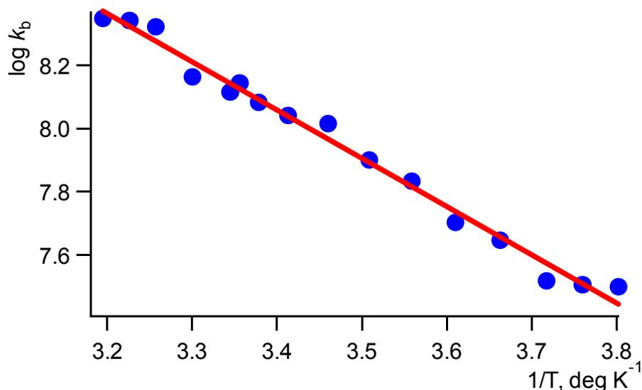
**Fig. 5.** Dependence of  $k_b$  vs. temperature in Arrhenius coordinates.
