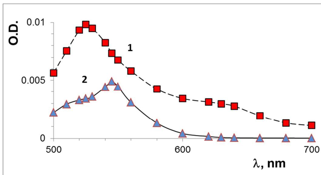
**Fig. 1.** Absorption spectra of transients in **E** film obtained at room temperature under laser flash photolysis of **B** in **E** with a delay after laser flash of: (1) 20 ns; (2) 0.5 ms. O.D. refers to optical density in this and subsequent Figures.
