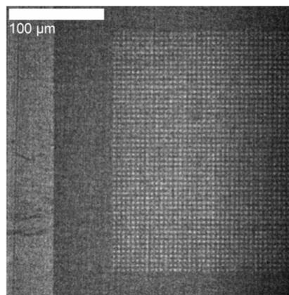
**Fig. 3.** Fluorescence microscopy image of zfRC-LH1 binding to DNA-functionalized glass surfaces. The DNA was patterned in a regular array of 2  $\mu\text{m}$  squares, defined by electron-beam lithography. Excitation: 532 nm. Emission: > 650 nm. The fluorescence signal on the left of the picture relates to a large marker in order to aid array location.
