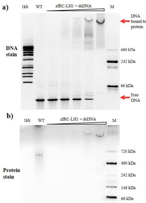
**Fig. 2.** Native gel electrophoretic analysis of zfRC-LH1 and stained for (a) DNA and (b) protein. zfRC-LH1 was incubated with 500nM 80bp DNA containing a single ZF binding sequence. 1kb: 1kb DNA ladder, WT: RC-LH1. zfRC-LH1 + dsDNA contains protein with an OD 0, 0.5, 1, 2.5 and 5. M: Nativemark protein marker (kDa). WT = wildtype.
