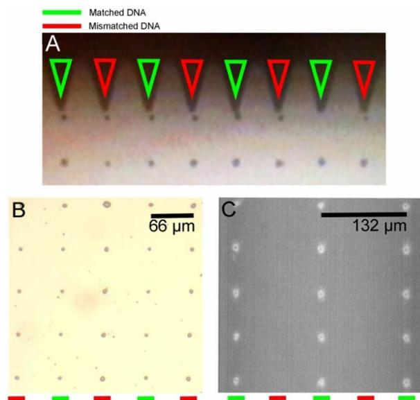
**Fig. 4.** Sequence-selective binding of zFRC-LH1 to matched and mismatched dsDNA using dual-sequence DPN. (a) DNA printing using pens to create alternate 5  $\mu\text{m}$  spots of matched (green) and mismatched (red) DNA. (b) Bright field image of the printed DNA array. (c) Fluorescence image of the pattern after ZF-RC-LH1 binding to DNA. Each row is spaced 66  $\mu\text{m}$  apart. Excitation: 532 nm. Emission: > 650 nm.
