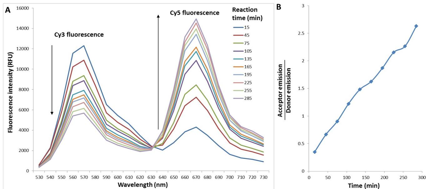
**Fig. 7** (A) Changes over time in the fluorescence spectrum ( $\lambda_{\text{exc}} = 460 \text{ nm}$ ) of Reaction 1 (see Table 1 for the reaction conditions). (B) Changes over time in the ratio of the emission at 670 nm (Cy5 emission) to the emission at 570 nm (Cy3 emission) in the fluorescence spectrum of Reaction 1 (see Table 1 for the reaction conditions).
