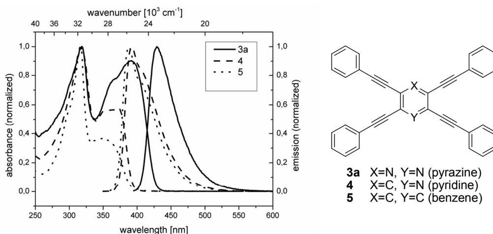
**Figure 3.** Comparison of absorption and fluorescence spectra of tetrakis(phenylethynyl)pyrazine **3a** with corresponding pyridine and benzene derivatives **4** and **5**, respectively.
