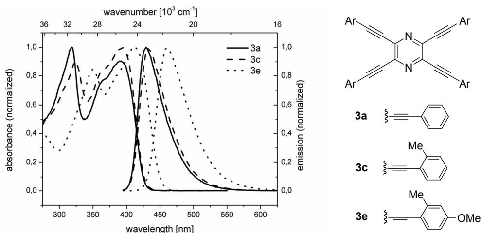
**Figure 2.** Normalized absorption and corrected emission spectra of compounds **3a**, **3c** and **3e** in CH<sub>2</sub>Cl<sub>2</sub>.
