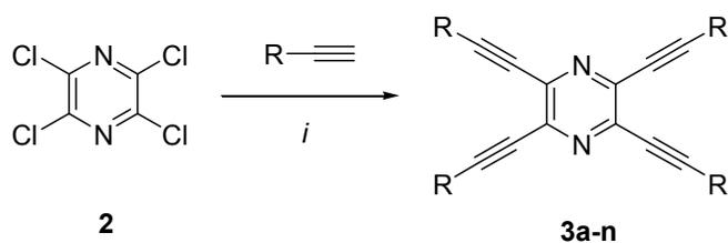
**Scheme 3.** Synthesis of **3a-n**; conditions: *i*: **2**, alkyne, PdCl<sub>2</sub>(CH<sub>3</sub>CN)<sub>2</sub> (3 mol%), X-Phos (6 mol%), CuI (5 mol%), HN(*i*Pr)<sub>2</sub>, 1,4-dioxane, 100 °C, 20 h.**Table 2.** Synthesis of **3a-n**.
