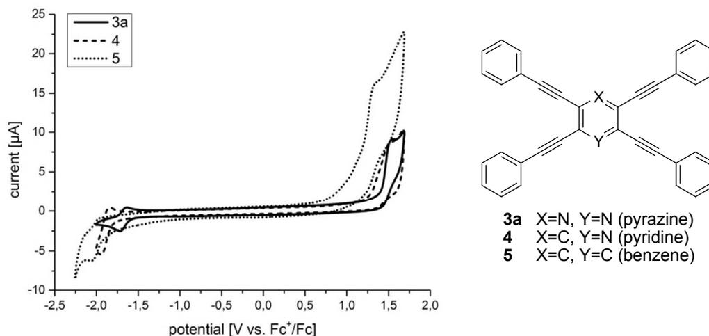
**Figure 4.** Cyclic voltammograms of tetrakis(phenylethynyl)pyrazine **3a** with corresponding pyridine and benzene derivatives **4** and **5**, respectively.
