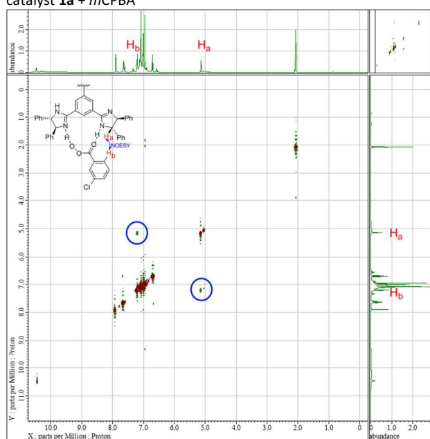
Fig. 3 2D-NOESY NMR spectrum of catalyst 1a and m CPBA in d^8 -toluene
