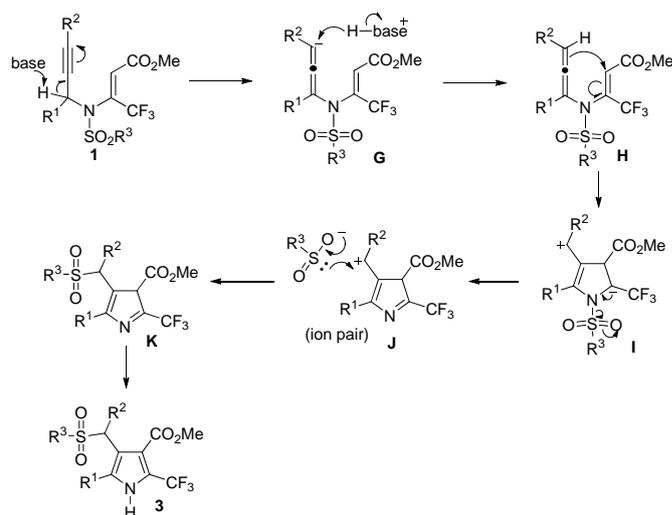
**Scheme 4** Proposed mechanism for the formation of pyrroles **3**.
