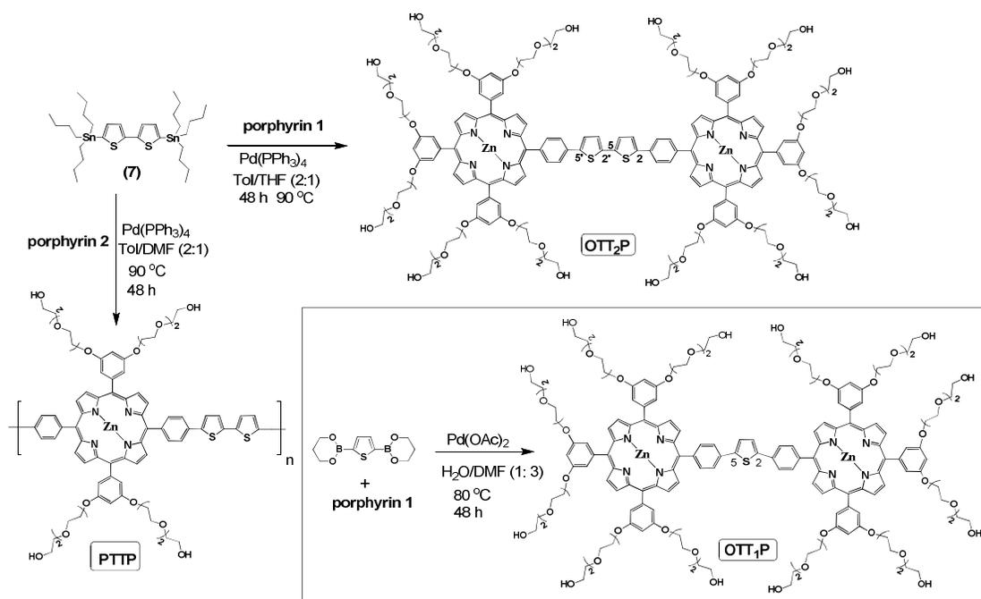
**Scheme 5.** Synthesis of Zn(II) oligo- and poly(2,5-thienylene)porphyrins.
