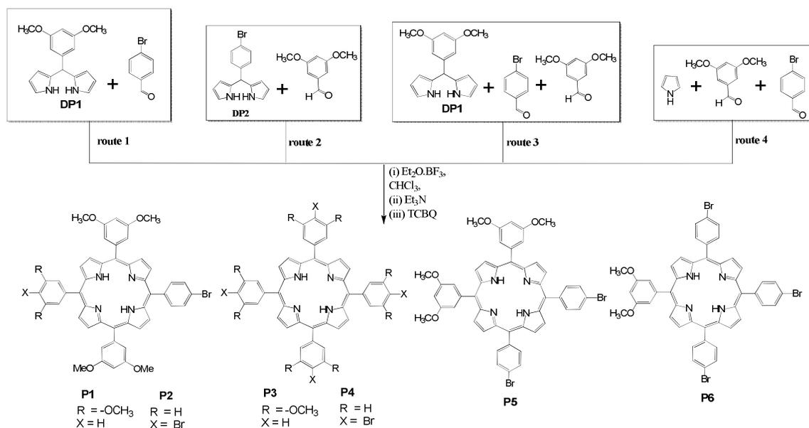
**Scheme 3.** Four different synthetic routes for the synthesis of porphyrin precursors.
