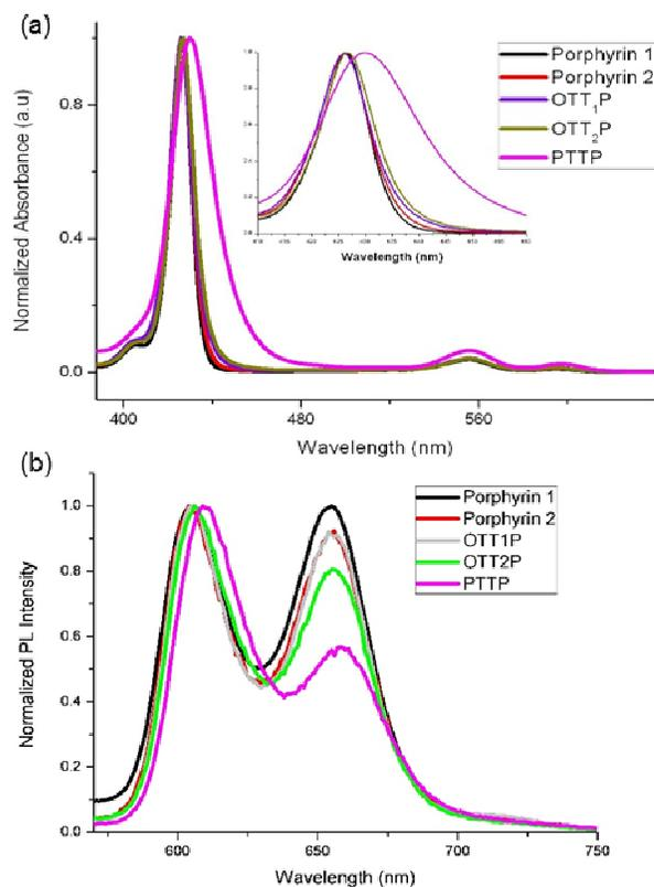
**Figure 1.** (a) Normalized absorption spectra of the compounds in  $\text{CHCl}_3$ . Inset of figure shows the focused version of the Soret band; (b) Normalized emission spectra of the compounds in  $\text{CHCl}_3$  ( $\lambda_{\text{exc.}}$  at 426 nm).
