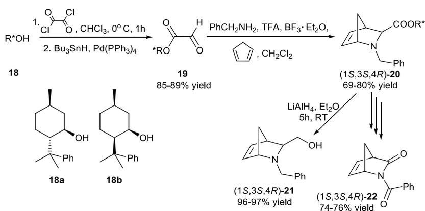
**Scheme 10.** Use of diastereomers of (-)-8-phenylmenthol **18a** and **18b** in the synthesis of 2-azanorbornene derivatives **21** and **22**<sup>31-33</sup>
