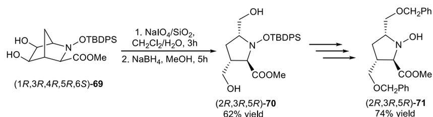
**Scheme 26.** Application of dihydroxylated 2-azanorbornene derivative **69** in the synthesis of functionalized pyrrolidines<sup>70</sup>
