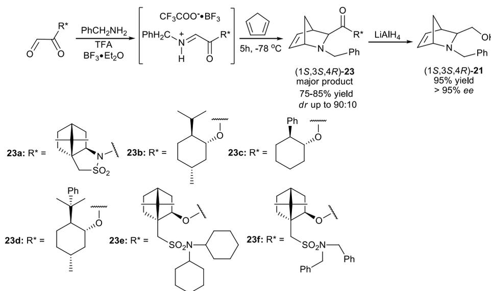
**Scheme 11.** Preparation of 2-azanorbornene derivatives **23** with the use of chiral auxiliaries
