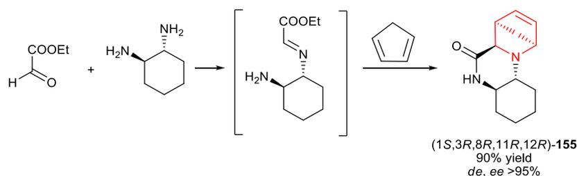
**Scheme 70.** Synthesis of the enantiopure tetracyclic compound using 1,2-diaminocyclohexane as a chirality source.<sup>163</sup> 2-Azanorbornene fragment in the tetracyclic product **155** indicated.
