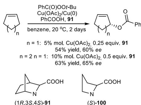
**Scheme 60.** Allylic oxidation of alkenes catalyzed by copper complexes<sup>127</sup>
