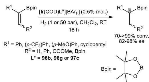
**Scheme 53** Asymmetric hydrogenation of unsaturated boronates<sup>117</sup>
