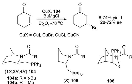
**Scheme 62.** 1,4-addition of a Grignard reagent to 2-cyclohexenone<sup>130</sup>
