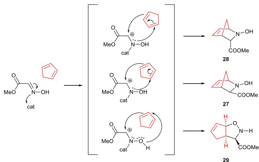
**Scheme 14.** Proposed mechanism for the cycloaddition of cyclopentadiene to oxime glyoxylate.<sup>41</sup>
