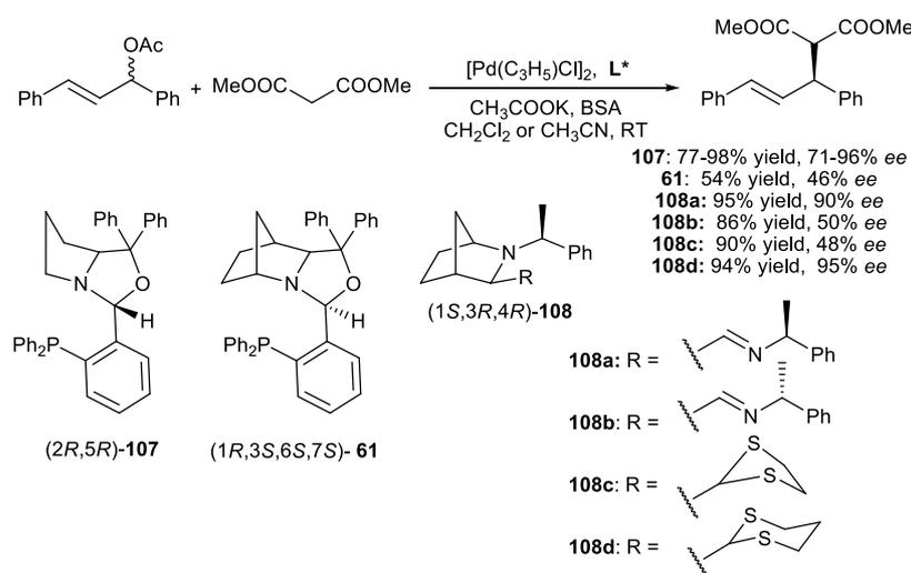
**Scheme 63.** Application of 2-azanorbornyl derivatives in palladium catalyzed AAA reaction.<sup>61,132</sup> Results for ligands **108** are given for 10% mol. of chiral ligand used.
