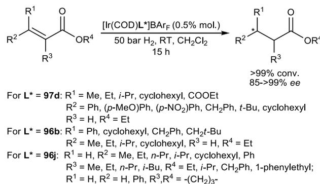
**Scheme 49.** Asymmetric hydrogenation of  $\alpha,\beta$ -unsaturated carboxylic esters<sup>112</sup>
