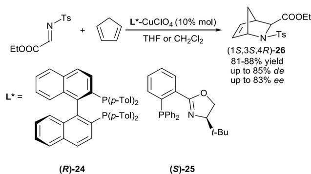
**Scheme 12.** Synthesis of 2-azanorbornene derivative catalyzed by a chiral copper(I) complex
