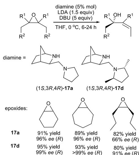
**Scheme 39.** Comparison of the efficiency of two chiral diamines in the rearrangement of *meso*-epoxides<sup>86</sup>
