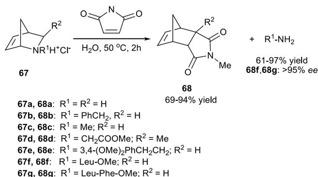
**Scheme 25.** Retro-DA reaction as a tool in the synthesis of chiral primary amines from 2-azanorbornenes<sup>67</sup>
