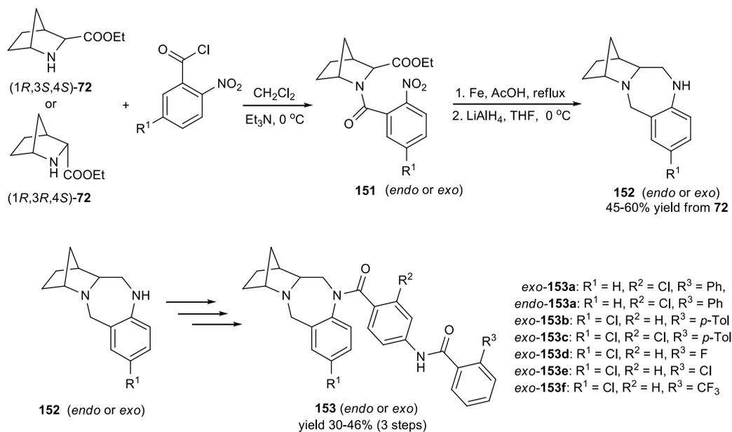
**Scheme 69.** Synthesis of benzodiazepines fused to a chiral 2-azanorbornane backbone<sup>161</sup>
