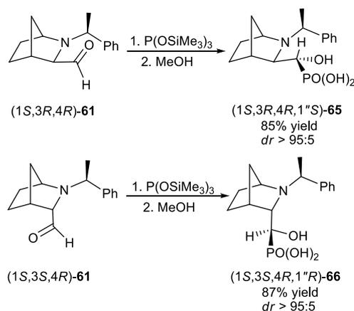
**Scheme 24.** Synthesis of  $\alpha$ -hydroxyphosphonic acids attached to a 2-azanorbornane<sup>66</sup>
