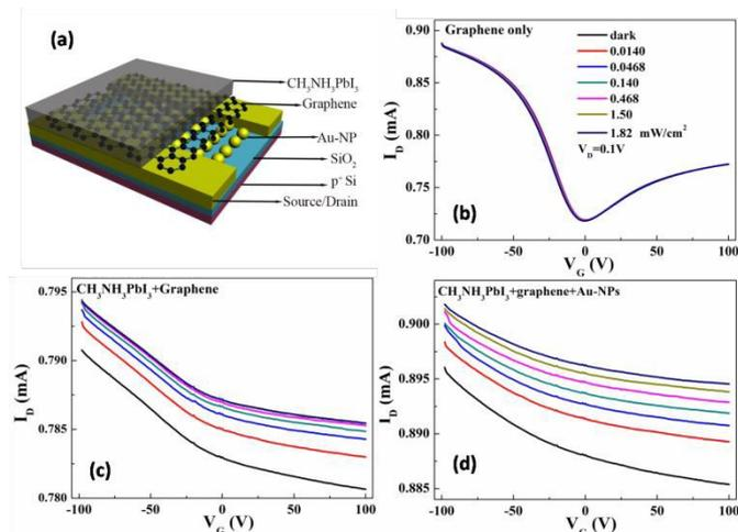
**Fig. 2** (a) Schematic of the device architecture used in this study. (b), (c) and (d) Transfer characteristics of the graphene-only,  $\text{CH}_3\text{NH}_3\text{PbI}_3$ -graphene (P-G), and  $\text{CH}_3\text{NH}_3\text{PbI}_3$ -graphene-Au-NPs (P-G-Au) device, respectively. These characteristics were measured under a  $V_{DS}$  bias of 0.1 V and under an illumination of a wavelength of 532 nm at different light intensities (listed in (b)).
