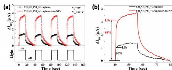
**Fig. 4** (a) The photo-switching characteristics of the P-G and P-G-Au devices under alternating dark and illumination conditions (wavelength = 532 nm, intensity =  $1.82 \text{ mW cm}^{-2}$ ). Dark time: 17s; light time: 23s. (b) Response time study on a single representative light/dark cycle.
