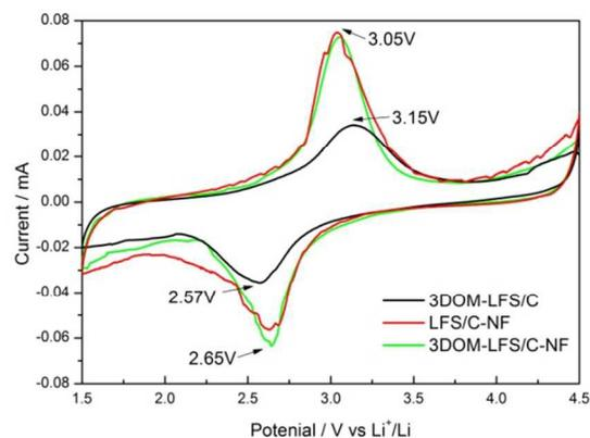
Fig. 7 Cyclic voltammetry (CV) of the 3DOM-LFS/C-NF compared with LFS/C-NF and 3DOM-LFS/C cathodes.
