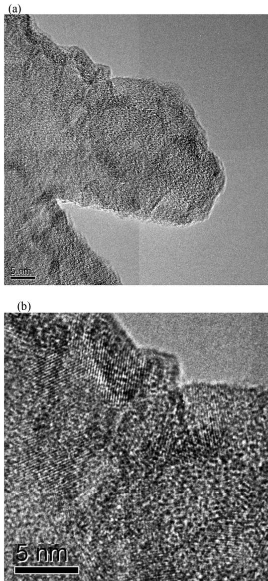
Fig. 4 TEM (a) and HRTEM (b) images of 3DOM-LFS/C-NF composites calcined at 650°C.
