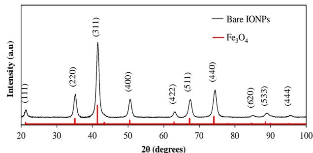
**Fig. 4** XRD pattern of IONPs. Peaks are indexed according to the reference pattern for magnetite (JCPDS PDF No. 00-019-0629).
