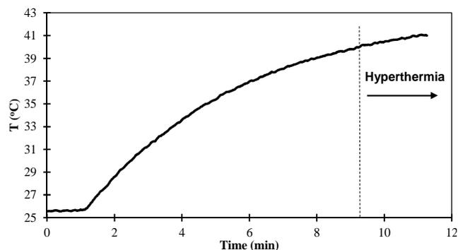
**Fig. 7** Typical heating curve of the MNCs dispersed in water with a concentration of 3 mg/mL and subjected to an AMF ( $f = 960$  kHz and  $H = 6.88$  kA/m).
