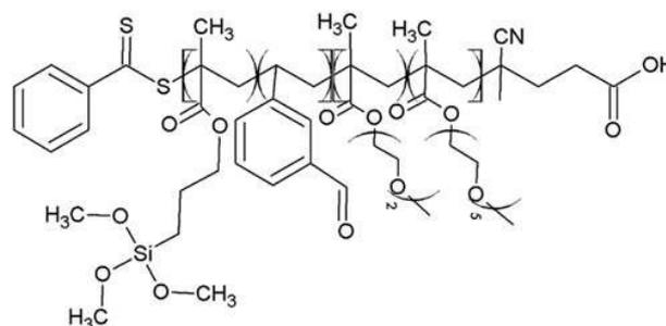
**Fig. 2** Chemical structure of P(DEGMA-*co*-PEGMA-*b*-[TMSPMA-*co*-VBA]) polymer.
