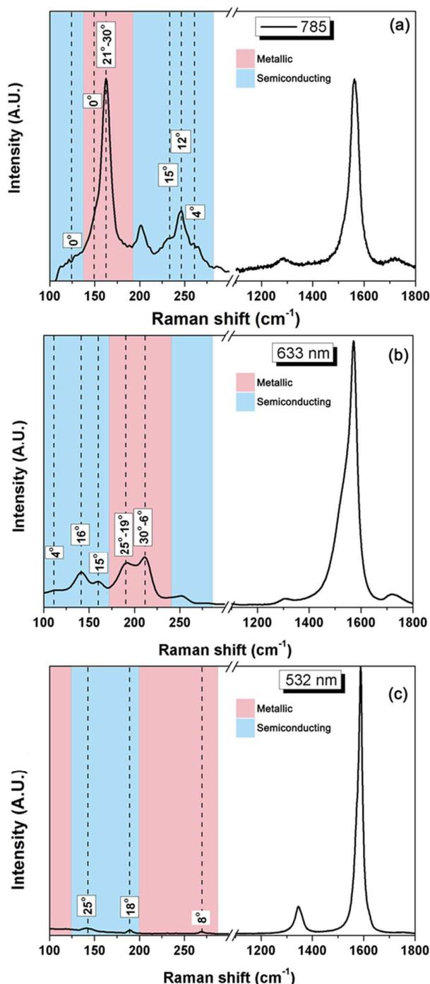
Fig. 2. CNT fiber Raman spectra acquired with (a) 785 nm, (b) 633 nm and (c) 532 nm lasers showing RBM Raman intensities, with apparent predominance of metallic SWNTs. Approximate chiral angles are indicated.
