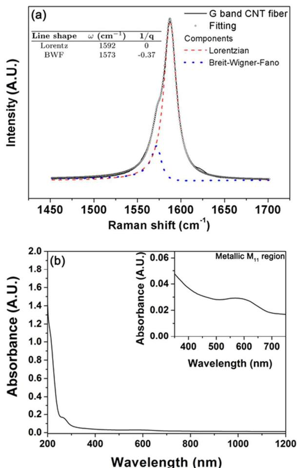
Fig. 3. (a) G band region of Raman spectra for CNT fiber showing the metallic line shape of the CNT fiber with a BWF asymmetric parameter  $1/q$  of  $-0.37$ . (b) UV-vis-NIR spectrum of a dispersion of the fiber constituent CNTs in  $\text{D}_2\text{O}$  solution with 1 wt.-% sodium dodecyl sulfate (SDS). The absorption spectrum shows the first-order transition from M SWNTs  $M_{11}$  (inset), but no absorption peaks from SC SWNTs.
