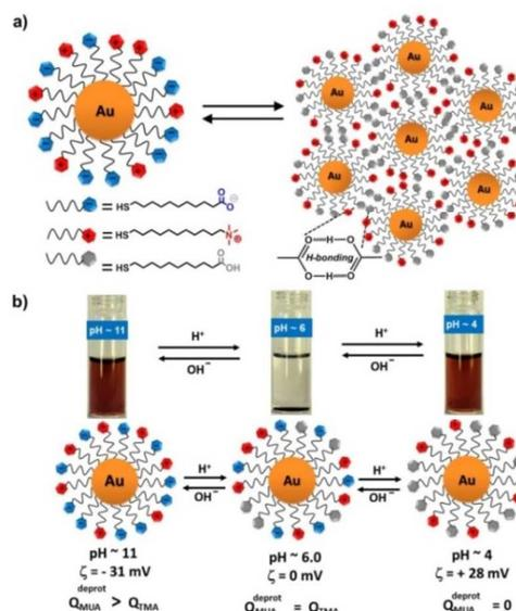
**Fig. 1** (a) Scheme of nanoparticles decorated with mixed SAMs comprising ligands illustrated in the legend. Crystals form when carboxylic acid groups are protonated and capable of hydrogen bonding. (b) Owing to the presence of both acidic and basic groups, the NPs are stable in water both at low and high pHs and precipitate only at the pH at which the net charge on the NPs is zero (see <sup>26</sup>).
