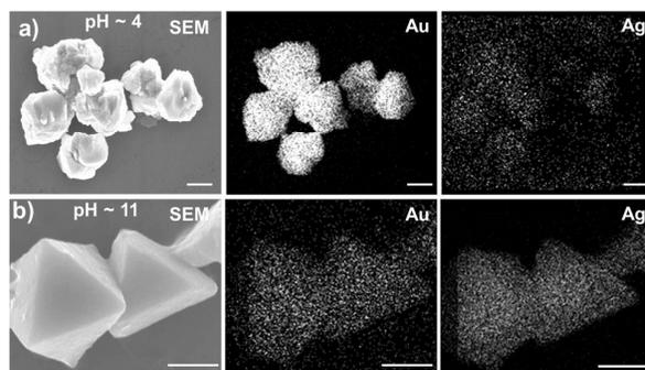
**Fig. 5** Characterization of crystals formed from mixtures of MUA/TMA AuNPs and TMA AgNPs at (a) pH  $\sim 4$  and (b) pH  $\sim 11$ , respectively. EDXS mapping confirms the presence of large quantities of Ag in crystals formed at pH  $\sim 11$ . Scale bar for (a) is 200 nm and for (b) is 1  $\mu\text{m}$ .
