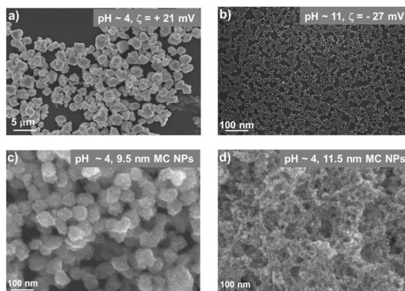
**Fig. 2** Four major types of structures observed for different particle sizes and different pH's: (a) smaller NPs (up to ca. 8 nm) form regularly faceted crystals at pH = 4; (b) unaggregated NPs are observed for all particle sizes at pH = 11; (c,d) non-crystalline aggregates are obtained from larger NPs at pH = 4.
