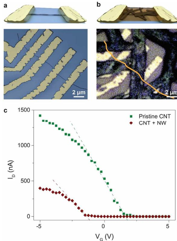
Figure 2: (a) Schematic representation and false color SEM micrograph of a series of a representative CNT-FET. (b) Schematic representation and optical micrograph of a representative  $MAPbI_3$ NW/CNT-FET. (c) Transfer characteristic in dark of a representative device before (green curve) and after (red curve) sensitization ( $V_D=0.2$  V). Dashed lines show the shift of the on-off threshold voltage  $V_{th}$ , and the reduction of the CNT mobility upon  $MAPbI_3$  deposition.
