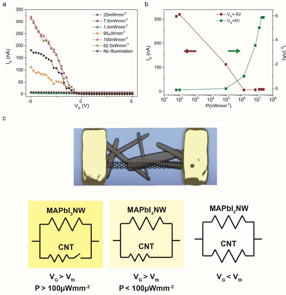
Figure 3. (a) Transfer characteristic of the hybrid phototransistor upon different light irradiation intensities. (b)  $I_D$  at  $V_G=5$  and  $-5$ V as a function of light power. (c) Schematic representation of the proposed two-parallel-resistor model used to describe our system.
