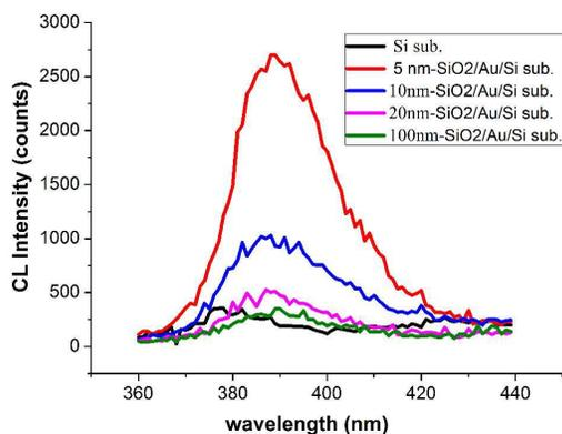
Fig. 4. UV peaks from the hybrid structure with  $\sim 500$  nm ZnO wires ( $h = 5, 10, 20,$  and  $100$  nm;  $E_0 = 10$  keV).
