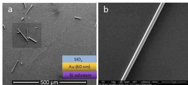
Fig. 1 SE images of the ZnO wires on the SiO<sub>2</sub> layer of the Au@SiO<sub>2</sub>/ZnO hybrid structure. (a) ZnO wires randomly distributed on the SiO<sub>2</sub> layer. Inset is the diagram of the plasmonic hybrid structure. (b) A ~500 nm ZnO wire on the SiO<sub>2</sub> layer.
