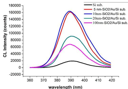
Fig. 3 UV peaks from the Au@SiO<sub>2</sub>/ZnO hybrid structure with ~1.6  $\mu\text{m}$  ZnO wires ( $h = 5, 10, 20,$  and  $100$  nm;  $E_0 = 10$  keV).
