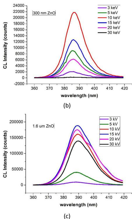
Fig. 8. NBE enhancement factor ( $R_{NBE}$ ) and NBE intensity ( $I_{NBE}$ ) vs. incident electron energy ( $E_0$ ): (a)  $R_{NBE}$  vs.  $E_0$  of  $\sim 300$  nm ZnO wires and  $\sim 1.6$   $\mu\text{m}$  ZnO wires from the plasmonic structure; (b) and (c)  $I_{NBE}$  vs.  $E_0$  of  $\sim 300$  nm and  $\sim 1.6$   $\mu\text{m}$  ZnO wires from the Si substrate ( $E_0 = 3, 5, 10, 15, 20$  and  $30$  keV,  $h = 5$  nm).
