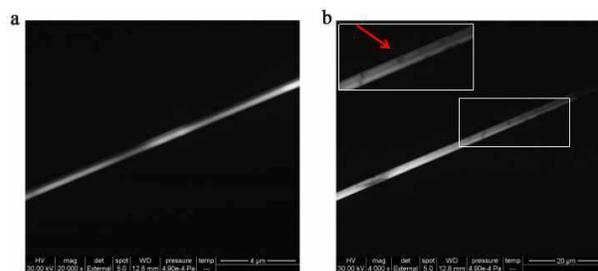
Fig. 6. Panchromatic CL images of ZnO wires in the plasmonic structures: (a) a  $\sim 300$  nm ZnO wire and (b) a  $\sim 1.6 \mu\text{m}$  ZnO wire.
