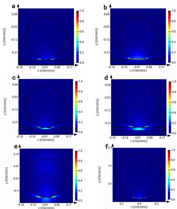
Fig. 7. FDTD simulations of the distribution of SPP field intensity ( $|E(x,y)|$ ) in the Au plasmonic hybrid structure in the  $x$ - $y$  plane. In the maps, black circles represent the profiles of the ZnO wires, and the two horizontal black lines represent the thickness of the  $\text{SiO}_2$  layer. The wavelength was 390 nm, and the thickness of the Au film was 60 nm. (a-e) a  $\sim 300$  nm ZnO wire with  $h = 2, 5, 10, 20$  and 100 nm. (f) a  $\sim 500$  nm ZnO wire with  $h = 5$  nm.
