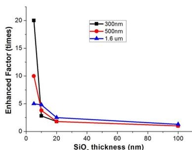
Fig. 5. Enhancement factors ( $R_{\text{NBE}}$ ) achieved with Au@SiO<sub>2</sub>/ZnO hybrid structures as a function of the thickness of the SiO<sub>2</sub> spacer and the diameter of the ZnO wires ( $h = 5, 10, 20$  and  $100$  nm;  $E_0 = 10$  keV).
