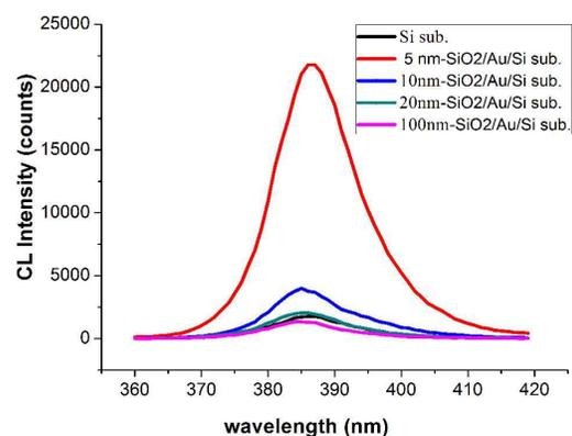
Fig. 2 UV peaks from the Au@SiO<sub>2</sub>/ZnO hybrid structure with ~300 nm ZnO wires, where the thickness of the SiO<sub>2</sub> spacer ( $h$ ) was 5, 10, 20, and 100 nm. The electron energy ( $E_0$ ) was 10 keV.
