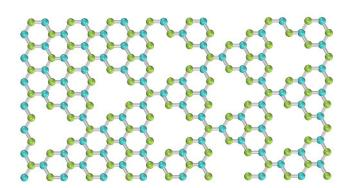
**Fig. 5** Graphene nitride nano sheet, riddled by triangular holes, was experimentally and computationally shown to exhibit an apparent piezoelectric response. Adapted from reference  $^{58}$ .
