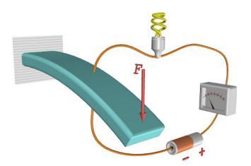
**Fig. 8** Schematic of a centrosymmetric flexoelectric energy harvester under base excitation. The cantilever beam is covered by conductive electrodes on its top and bottom surfaces. Due to application of an external force or the movement of the base, the cantilever beam undergoes bending vibrations. Due to flexoelectric contribution, an alternating potential difference is generated across the electrodes. Adapted from reference<sup>79</sup>.
