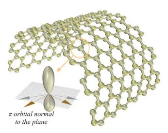
**Fig. 2** Bending of graphene: upon bending, the symmetry of the electron distribution at each atomic site is broken, which leads to the polarization normal to the graphene ribbon; an infinite graphene sheet is semi-metallic; however, finite graphene nanoribbons can be dielectric depending upon surface termination. Adapted from reference  $^{29}$ .
