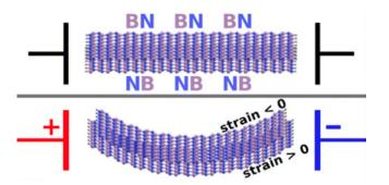
**Fig. 3** Duerloo and Reed<sup>53</sup> found that a bilayer consisting of two BN monolayers exhibits a strong curvature induced electromechanical coupling. Using quantum mechanical calculations and a continuum model, they found that these bilayers (in response to an external electric field) amplify in-plane displacements by factors of as much as  $10^3 - 10^4$ —when compared with a single monolayer. Reproduced with permission from reference.<sup>53</sup>
