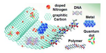
Fig. 6 Chemical doping of graphene surface with different components such as Nitrogen, polymers, and various metals can induce a piezoelectric response. Reproduced with permission from reference  $^{64}$
