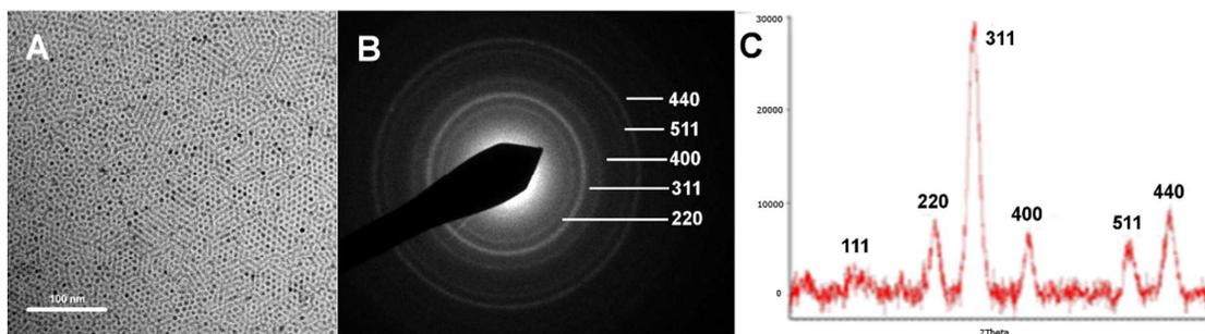
**Figure 1.** **A**, TEM micrograph of as-prepared  $\text{Fe}_3\text{O}_4$  nanoparticles (oleic acid capped). **B**, SAED showing  $\text{Fe}_3\text{O}_4$  lattice ring patterns. **C**, XRD diffractogram with indexed peak positions. Scale bar, 100 nm.
