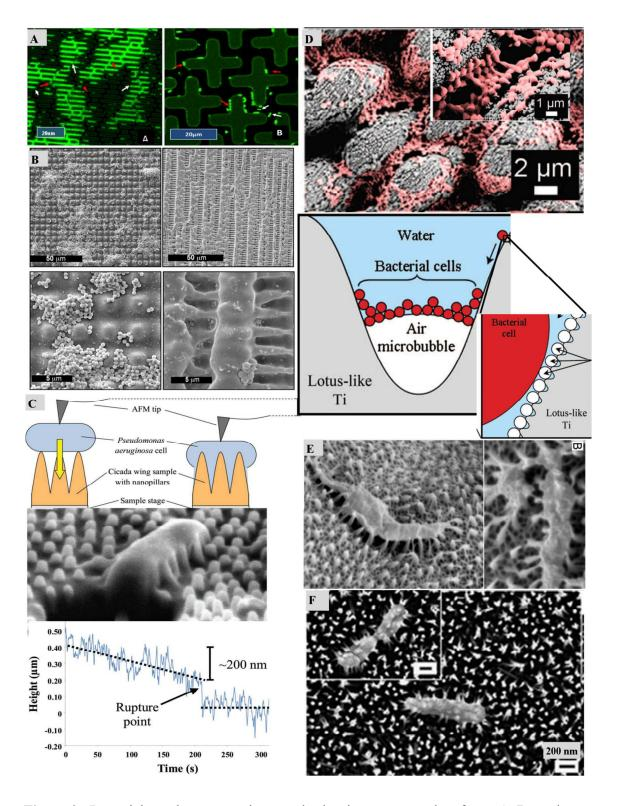
**Figure 2.** Bacterial attachment on micron and sub-micron patterned surfaces. **A**, Bacteria are attached on the micropatterned surface which mimics the riblet-like patterns present of the shark skin (left) and on the cross-patterns (right), reproduced with permission from Ref <sup>34</sup>. **B**,
