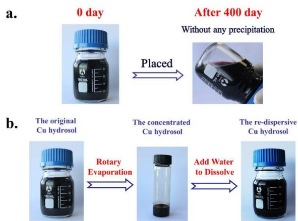
Fig. 3 a) The nano Cu hydrosol of freshly prepared and after placing for 400 days; b) The original nano Cu hydrosol after concentration and re-dispersion.
