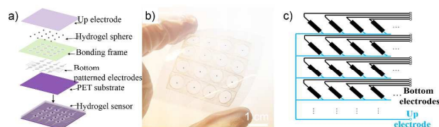
Fig. 2 The skin-like pressure sensor. a) The fabrication process, b) a photograph of the sensor and c) the schematic equivalent electric circuit.
