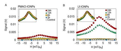
Fig. 5. MPS signals and their normalized data (inset) of C6 cells in DMEM medium (control), (A) C6 cells after incubation with PMAO-IONPs for 2, 6, 12, and 24h, and (B) C6 cells after incubation with Lf-IONPs for 2, 6, 12, and 24h. Higher signal intensities were observed for C6 cells incubated with Lf-IONPs compared to those with PMAO-IONPs. FWHM remained the same between incubation time of 6 to 24h.
