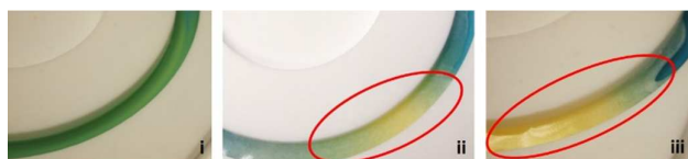
Figure 5. Close-up pictures showing portion of the system containing pre-mixed solutions with (i) 0.75 \times 10^4 , (ii) 2.25 \times 10^4 and (iii) 4.50 \times 10^4 propelling micromotors. Formation of a layer of bubbles on top of the solution are circled in red. The photographs were taken following the addition of NaOH pellet at the bottom of the system, at 5 minute mark for (i) and at 10 minute mark for (ii) and (iii). Width of channels = 1 cm.
