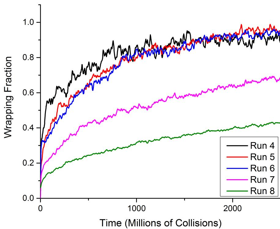
**Figure 4:** The wrapping fraction as a function of time for nanoparticles with diameters of 20 $\text{\AA}$  (Run #4), 40 $\text{\AA}$  (Run #5), 40 $\text{\AA}$  (Run #6), 60 $\text{\AA}$  (Run #7) and 100 $\text{\AA}$  (Run #8). The nanoparticle mass densities were 0.01 amu/ $\text{\AA}^3$  for Run #4, #5, #7 and #8 0.13 amu/ $\text{\AA}^3$  for Run #6. The time is displayed as the time in millions of collisions.
