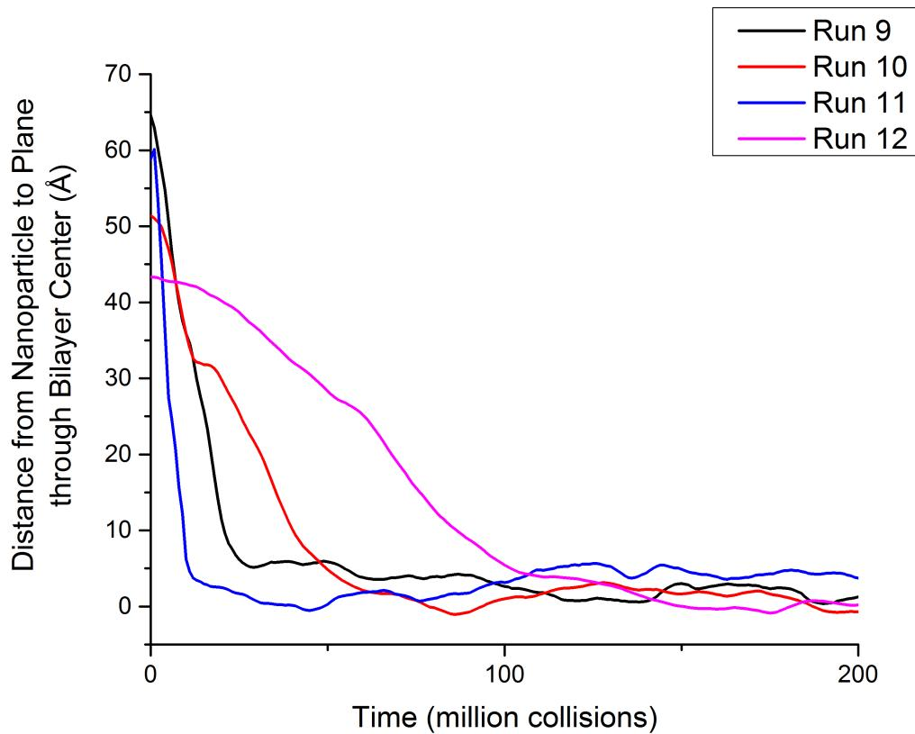
**Figure 7:** The distance from the nanoparticle to the plane through the bilayer center for runs #9, #10, #11 and #12. The zero time point for each run is set to the time when the nanoparticle first has a square-well interaction with a lipid tail coarse-grained site.
