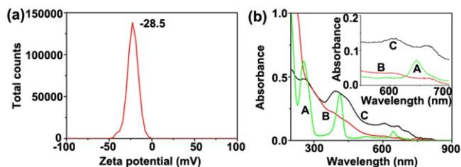
**Fig. 2** (a) Zeta potential distribution of  $\text{MoS}_2$  nanoplates. (b) UV-vis-NIR spectra of (A) Ce6-aptamer, (B)  $\text{MoS}_2$ , (C) nanoprobe. Inset: the absorbance of A, B, C in the wavelength range of 550 to 700 nm.
