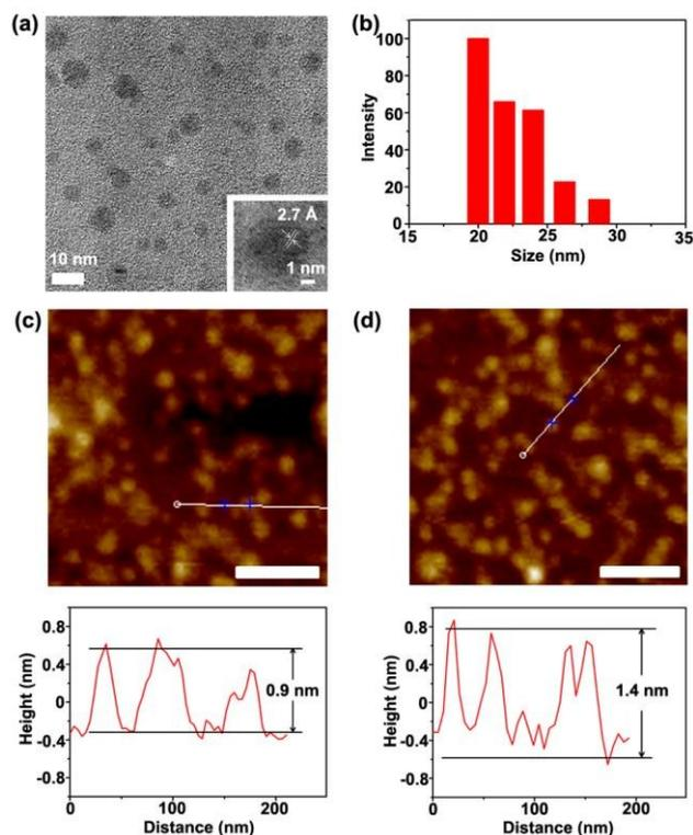
**Fig. 1** (a) HRTEM image of  $\text{MoS}_2$  nanoplates. Inset: HRTEM image highlighting the 2.7-Å lattice fringes that correspond to the (100) planes. (b) DLS characterization of the prepared  $\text{MoS}_2$  nanoplates. AFM characterization of (c)  $\text{MoS}_2$  and (d) nanoprobe, and the corresponding height images. Scale bar: 100 nm.
