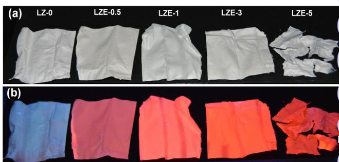
**Fig. 5** Photographs of LZ-0, LZE-0.5, LZE-1, LZE-3, and LZE-5 nanofibrous membranes. (a) The pictures were taken under white light. (b) The pictures were taken in a dark room by using a 254 nm ultraviolet lamp as excitation source.
