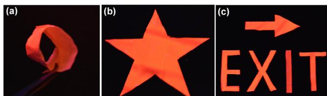
**Fig. 9** Luminescent photographs for LZE-3 nanofibrous membranes. The pictures were taken in a dark room by using a 254 nm ultraviolet lamp as excitation source. (a) Photograph depicting the mechanical softness of LZE-3 membranes. (b) The “Pentagram” pattern. (c) The “EXIT” pattern.
