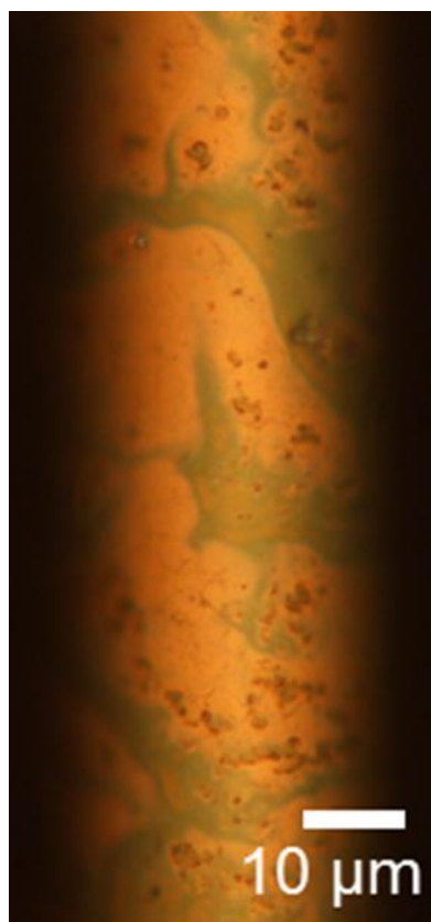
Figure 2. Dark-field optical microscope image of drawn-capillary OFRR with C8 MPN coating showing the non-uniformity of the C8 MPN film.
