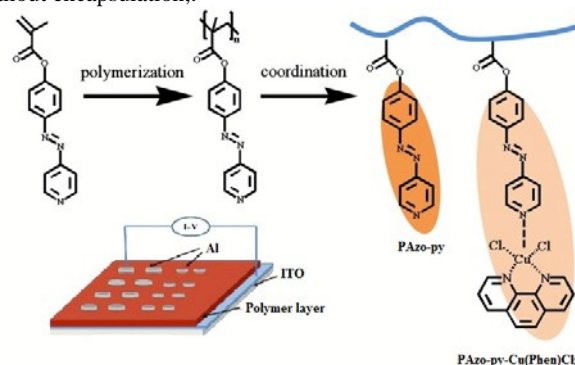
Figure 1. Synthetic routine of PAzo-py and PAzo-py-Cu(Phen) \text{Cl}_2 .
