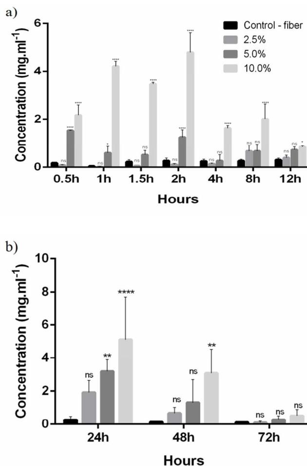
**Fig. 3** Cm-p1-PVA release analyses from nanofibrous membranes (a) using different scaffolds in hours and (b) from the same scaffolds until 72 hours. NS: no significance. (\* $P < 0.1$ ; \*\* $P < 0.01$ ; \*\*\*\* $P < 0.0001$ ).
