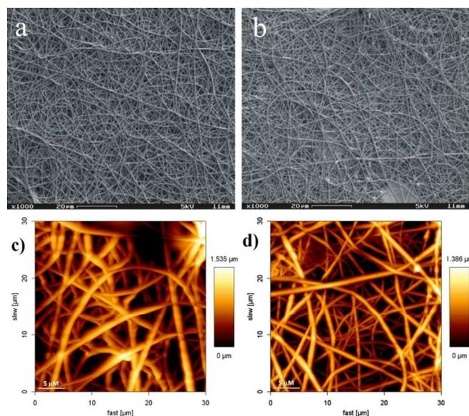
**Fig. 2** SEM and AFM micrographs of PVA and Cm-p1-PVA fibers. (a) 10 % PVA fibers in 1000x magnification by SEM, (b) 10 % Cm-p1-PVA fibers in 1000x magnification by SEM, (c) 10 % PVA fibers by AFM and (d) 10 % Cm-p1-PVA fibers by AFM.
