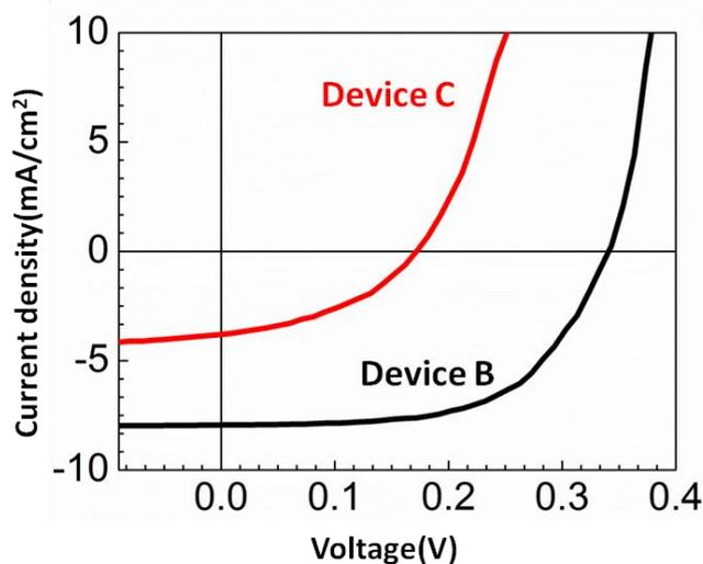
Figure 6 Light current density-voltage ( $J$ - $V$ ) plots of single wire  $p^+-n^+$  junction Si nanowire devices with different  $n$ -type shell layer coating measured under 1-sun illumination.
