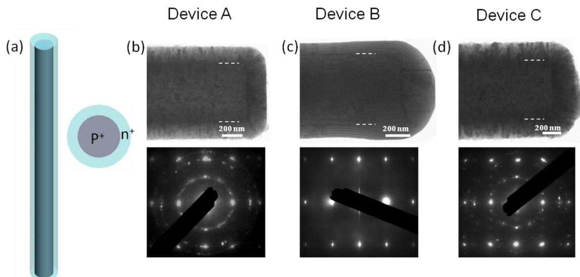
Figure 1 (a) Schematics of the core/shell ( $p^+/n^+$ ) silicon nanowire structure. TEM images (top) and corresponding electron diffraction patterns (bottom) of diodes fabricated with (b)  $650^\circ\text{C}$   $n$ -type Si shell layer coating (Device A); (c)  $950^\circ\text{C}$   $n$ -type Si shell
