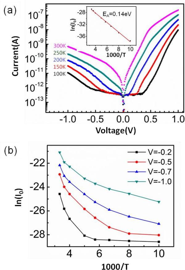
Figure 5 (a) Semi-log plot of variable temperature  $I$ - $V$  curves of 950°C annealed 650°C coated single wire device (Inset: Arrhenius plot of  $\ln(I_0)$  versus  $1000/T$ ). (b) Arrhenius plot of current as a function of temperature at bias  $V = -0.2, -0.5, -0.7$  and  $-1V$
