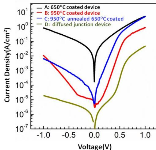
Figure 3 Semi-log plots of the dark current density-voltage (*J*-*V*) curves of the *p*<sup>+</sup>-*n*<sup>+</sup> junction devices fabricated with *n*-type Si shell layers deposited by LPCVD under different conditions. The *J*-*V* curve from a diffused *p*<sup>+</sup>-*n*<sup>+</sup> radial junction microwire (diameter of 8μm) array device is included for comparison.
