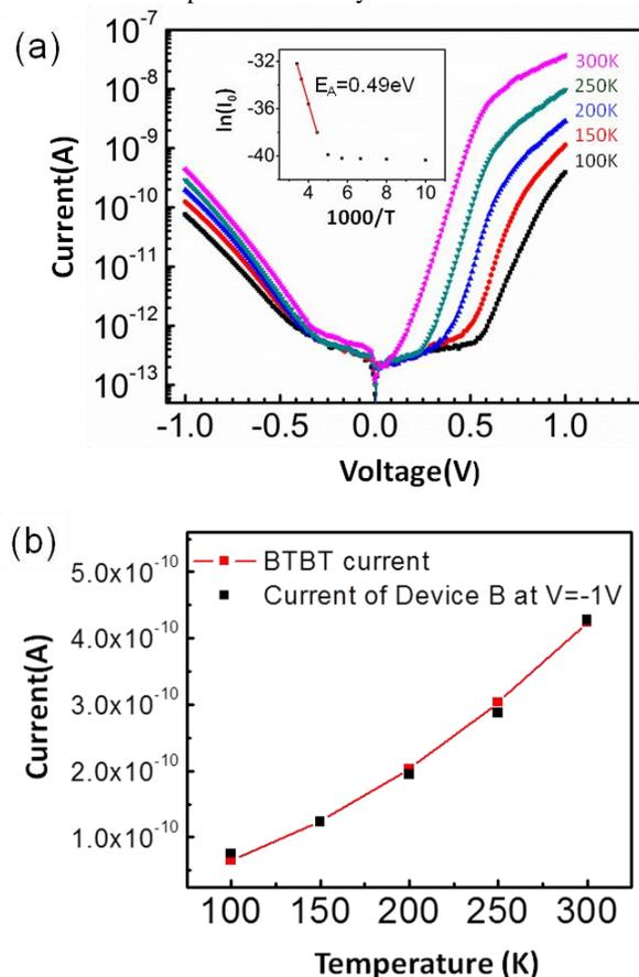
Figure 4 (a) Semi-log plot of variable temperature  $I$ - $V$  curves of 950°C coated single wire device (Inset: Arrhenius plot of  $\ln(I_0)$  versus  $1000/T$ ). (c) Current at bias  $V = -1V$  as a function of temperature. The red line with symbols is the calculated current using the BTBT current model and  $-1V$ .
