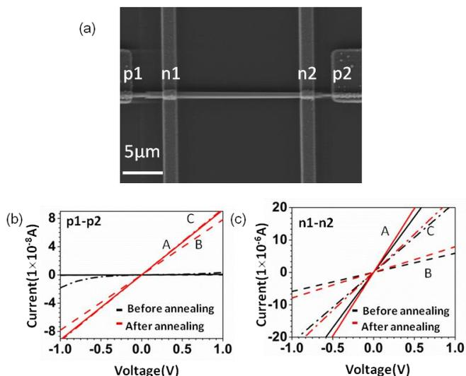
Figure 2 (a) FESEM image of a single nanowire device with four Ti/Pd contacts. p1 and p2 are in contact with *p*-type core, n1 and n2 are in contact with the *n*-type shell. Current-voltage (*I*-*V*) curves obtained across electrodes p1-p2 (b) and n1-n2 (c) of different types of devices.
