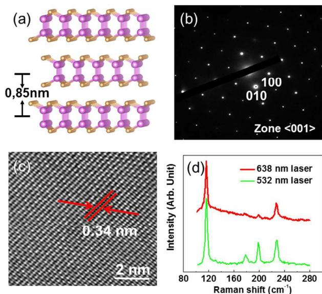
Figure 1. (a)  $\epsilon$  polytype crystal structure of InSe with the  $c$ -axis vertical. Orange and purple spheres represent Se and In atoms respectively. (b) TEM SAED pattern of 10-layer InSe with the beam parallel to the  $c$  axis (c) The corresponding HR-TEM of InSe on a holey carbon grid with the lattice spacing of 0.34 nm. (d) Raman spectra of 12-layer InSe on  $\text{SiO}_2/\text{Si}$  substrate.
