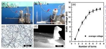
**FIG. 2** (a-b) The electrospinning process by using the SPEA; (c) Optical microscope image of the PS fibers; (d) 3D stacking structure of PS fibers. (e) The relationship between the number of turns and the generated static voltage between needle and collector of the SPEA.
