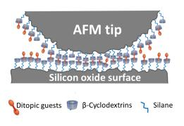
Fig. 1 Schematic representation of a  $\beta$ -CD hosts monolayer attached to an AFM tip and silicon wafer. Hydrophobic interactions lead to inclusion of the connector molecules into the hosts and to the tip-sample interaction.
