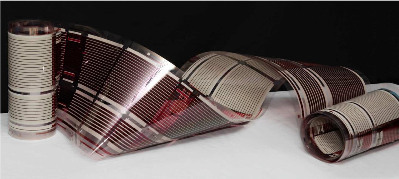
Figure 5. R2R fabricated printed inverted OPV modules using gravure printing and rotary screen printing techniques.
