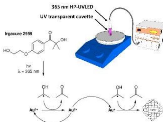
**Fig. 1** AuNPs photochemical synthesis in the presence of Irgacure® 2959 using UV LED irradiation system (365 nm, 350  $\text{mW}\cdot\text{cm}^{-2}$ ).
