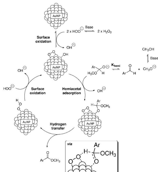
Fig. 10. Schematic mechanisms of the reaction pathways in the photocatalytic oxidative esterification of aromatic aldehydes by AuNPs/PTFE in the presence of  $H_2O_2$  and a strong base.
