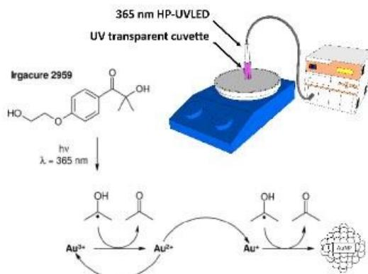
Fig. 1 AuNPs photochemical synthesis in the presence of Irgacure® 2959 using UV LED irradiation system (365 nm, 350 mW.cm<sup>-2</sup>).
