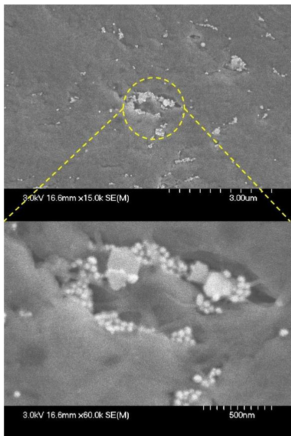
**Fig. 4** SEM analysis of the PTFE immobilized AuNPs surface.
