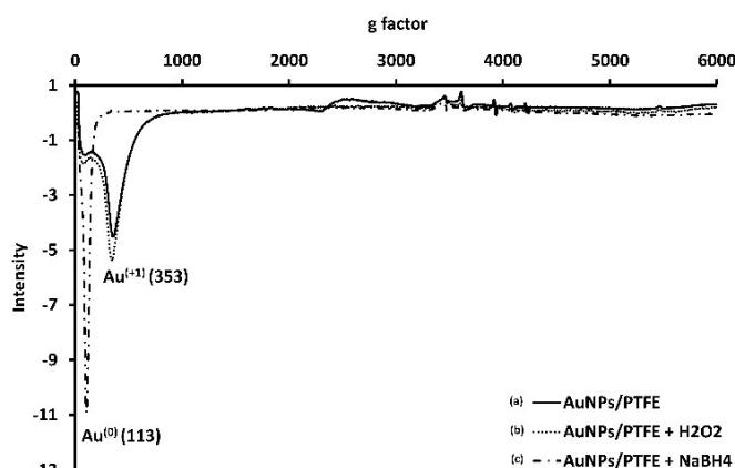
**Fig. 6** AuNPs/PTFE EPR (5 K) spectra.
