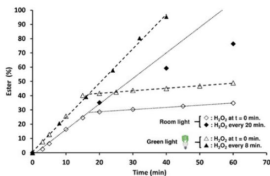
**Fig. 7** Kinetic of benzoic acid methyl ester formation. Comparison between standard (◇), photocatalyzed (△), standard with repeated H<sub>2</sub>O<sub>2</sub> additions (◆) and photocatalyzed with repeated H<sub>2</sub>O<sub>2</sub> additions (▲) conditions.
