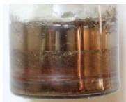
**Figure 1.** Detail of a metallic mirror deposited on a glass reactor under multiphase conditions
