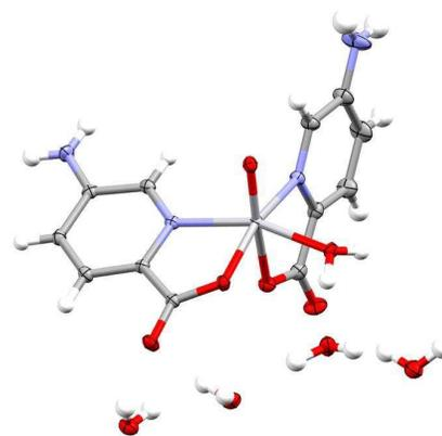
**Figure 2.** Perspective view of the mononuclear entity of compound **2**. Thermal ellipsoids are drawn at the 50% probability level. Color code: N = blue, O = red, C = grey, V = grey-blue.
