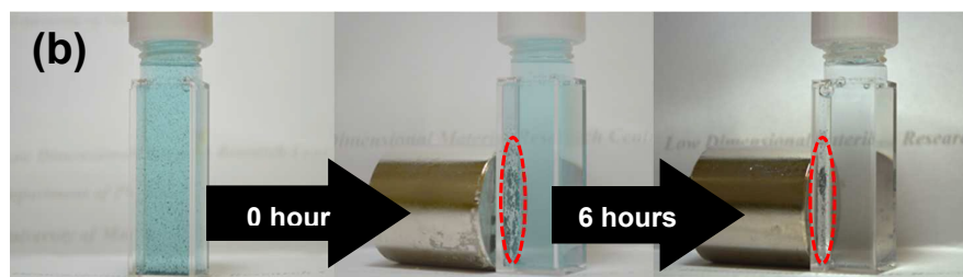
803 Fig. 13 (a) Recyclability of magnetic photocatalytic degradation of MB in the 804 presence of \text{CoFe}_2\text{O}_4 decorated 3D \text{TiO}_2 magnetic nanocomposite. (b) 805 Magnetic photocatalytic \text{CoFe}_2\text{O}_4 -3D \text{TiO}_2 nanocomposites were recovered 806 from the treated MB solution. The composite is set for magnetic separation 807 after 6 consecutive hours of irradiation and could be reused several times 808 without any significant loss of magnetic responsiveness and photocatalytic 809 reactivity.
