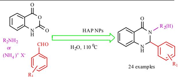
HAP NPs were applied as a green heterogeneous catalyst for synthesis of 2,3-dihydroquinazolin-4(1*H*)-one derivatives.
