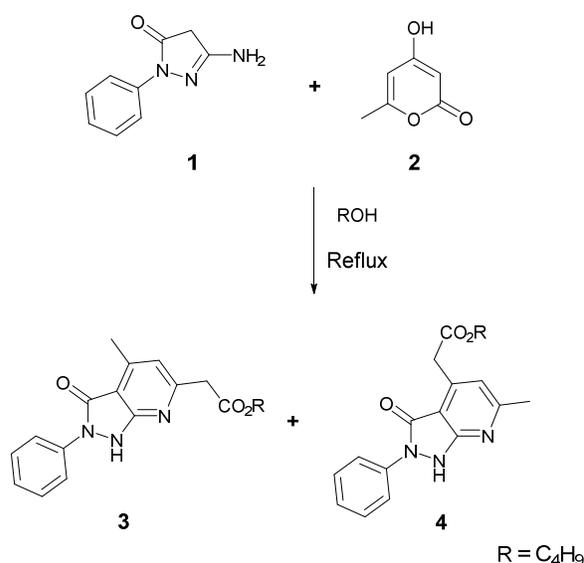
**Scheme 1** Synthetic route to pyrazolo[3,4-b]pyridines from condensation of 3-amino-1-phenyl-2-pyrazolin-5-one **1** with 4-hydroxy-6-methylpyran-2-one **2**
