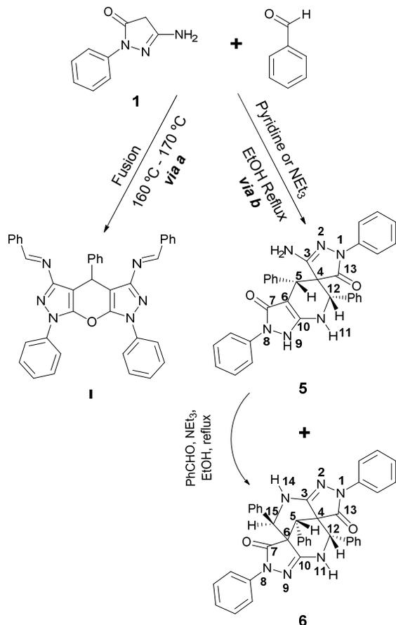
**Scheme 2** Reactivity of 3-amino-1-phenyl-2-pyrazolin-5-one **1** with benzaldehyde under different experimental conditions
