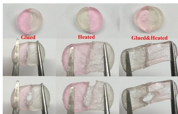
Fig. 3. The stretching of the hydrogels with different healing process.
